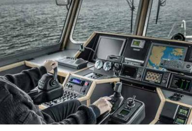
The buttons on the joystick put a unique combination of functions within your easy reach. Dynamic Positioning, Joystick Driving, Joystick Docking and High Mode offer easier handling, increased safety, and reliable operation.
