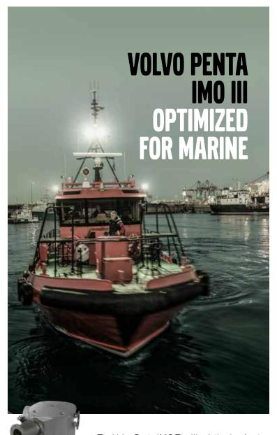
Proven SCR technology ensures high engine power output while offering efficient NOx reduction. The Volvo Penta IMO Tier III solution is robust and designed for tough marine conditions. Based on SCR exhaust aftertreatment technology, our solution is available for IPS, inboard, genset and auxiliary applications. It is designed for flexibility, ease of installation and space-efficient configuration.
